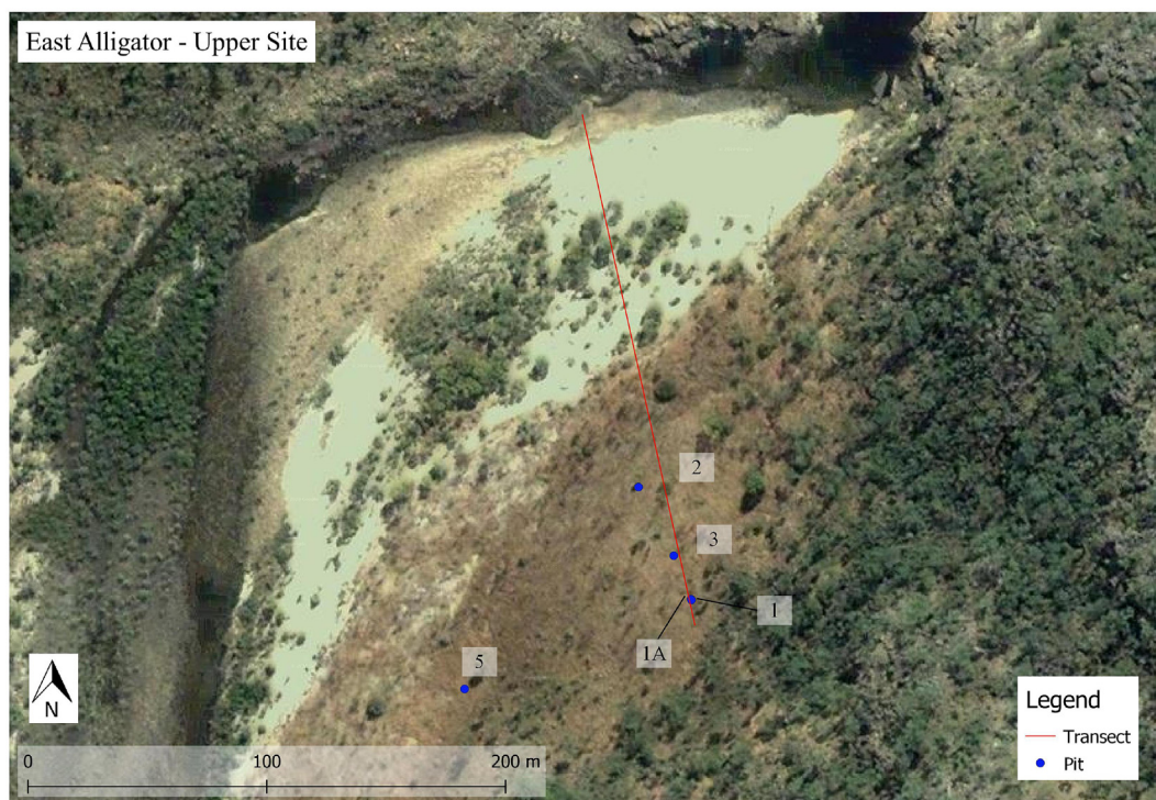
Fig. 2. Satellite image from Google Earth™ showing the main features of the upstream slackwater site, the survey line for palaeodischarge calculations, and the locations of the pits in the alluvial deposits. Flow is from left to right.
