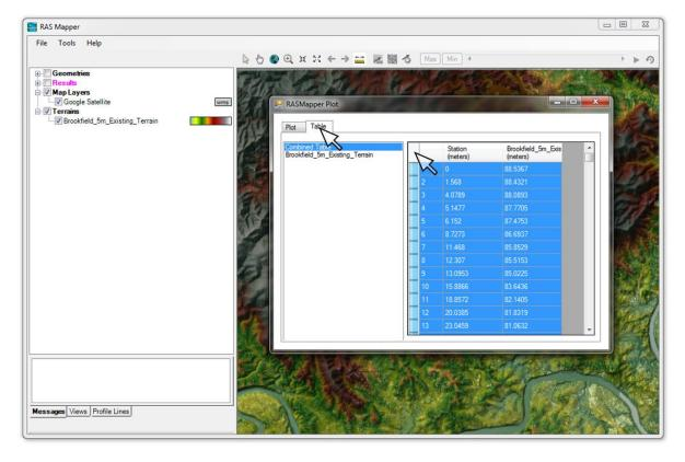
• Repeat the process by selecting the measuring tool, but this time click on "Save as Profile Line" and enter a name for the profile line.
